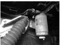
Secure the fuel pipes against the chassis ensuring that you don't stress the pipes as the plastic ends can get damaged easily.
