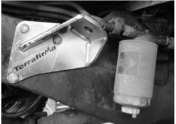
With TF519 top shock mount fitted as pictured left remove the bolts securing both filter housing and backing plate from the chassis, using the M8 countersunk bolts bolt the relocation plate on to the chassis using the aluminium spacers to allow the plate to stand proud.
