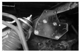
Discard the tin backing plate and using the original bolts remount the filter head to the plate using the top two holes. If necessary slacken and adjust the top shock mount position to allow more clearance around the fuel pipes.
