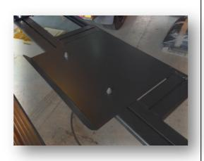
2. Using the access slots slide the leg mounting bolts into position.
