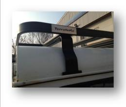
Only when you are happy with the position tighten the gutter clamps evenly taking care not to over tighten. Finally tighten all the leg mounting bolts.
