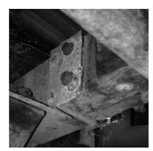
Mount the R/H plate (with return pointing inward) this mounts using the lower bumper bolt and the front upper steering box bolt. (See photo left)
