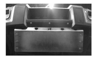
Finally you need to secure the lower valance there are two ways to do it one is to use a drill with an 8mm socket attachment and simply drill the screw through the blade or if you don't have that facility then drill a 3mm hole through the guard and then drive the self-drilling screws through the plate with the ratchet and 8mm socket.
