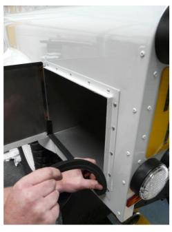
Due to the thickness of the rubber seal used to prevent water and dust ingress into the locker the door will require force to close initially, this should get a little easier after time.
