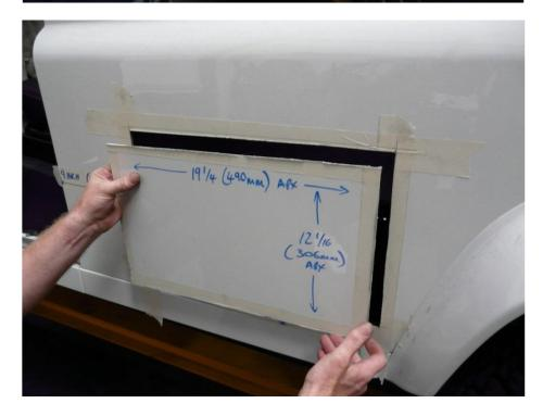
Once you have measured and checked, measured and checked again and you are happy an ultra-thin metal cutting disc is recommended, but take extra care at the corners and be careful of the heat generated.
