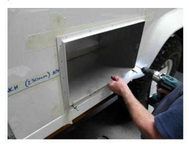
Some fitters like to use a small amount of bond between the mating surface's, should you wish to do the same please use a suitable bond compatible with all materials.
