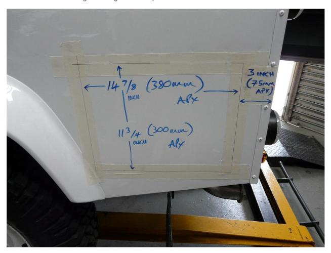
The key to fitting the rear locker is masking tape, a ruler, tape measure and a pen. You can accurately measure out where you want to cut the vehicle and check the box and cut lines for a tight fit and for square.
