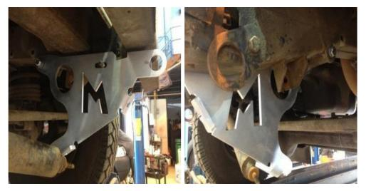
Offer up the front guard to the two side brackets and bolt together but do not tighten yet.
