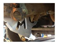
Please note that there is only 1 x M10 x 110mm bolt in the fitting kit. There's a long bolt on the driver's side of the vehicle that secures the steering box bracket to the chassis, this is the bolt that secures the steering guard mounting arms to the chassis, the long bolt in the fitting kit does the same job on the passenger side.
