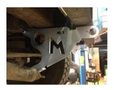
Pass the steering damper through the hole and re-bolt to the chassis.
