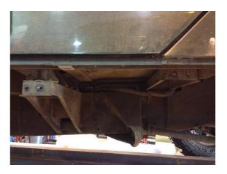
making sure the rock slider is level with body work, re-tighten the bulkhead bolts to the land rover recommended torque settings.
