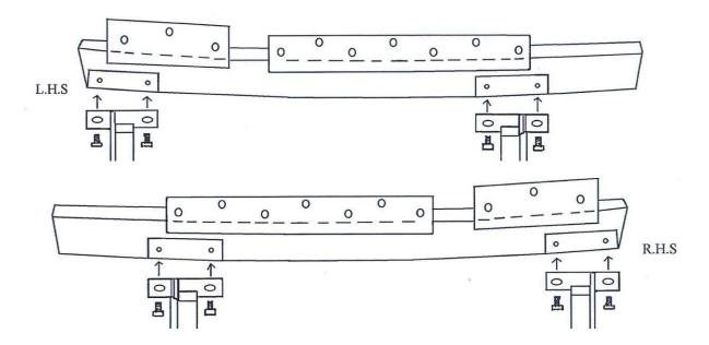
After the Rock Sliders have been mounted check all nuts have been fully tightened.
