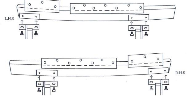
After the Rock Sliders have been mounted check all nuts have been fully tightened.
