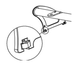
Offer the bar up to the holes you just drilled. Push one of the M6 button head screws with a washer through the rear hole and screw it carefully into the rear most nut in the bar. This will hold the bar in place so next do the same on the other side then the two fronts.
