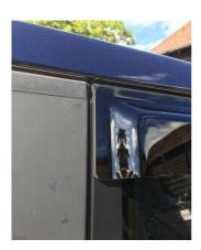
Rear deflectors should align perfectly with the door frame.
