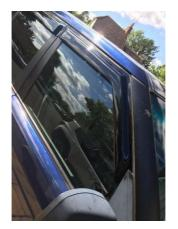
Ensure the right angle on the deflector meets the right angle of the mirror mounting.
