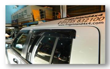
Rear deflectors should align perfectly with the door frame.
