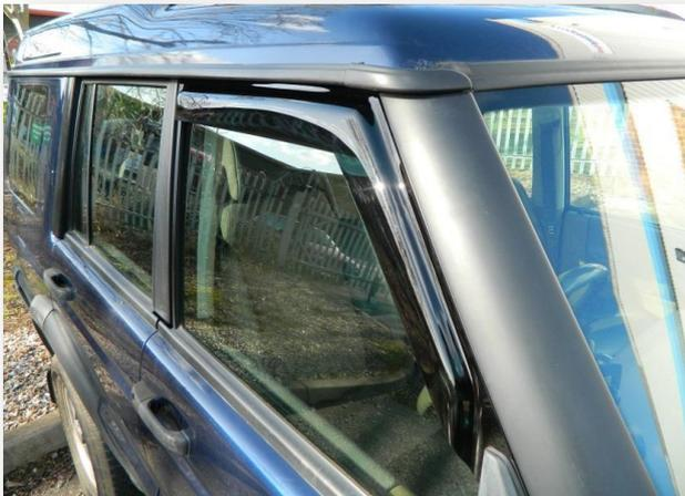
Ensure the right angle on the deflector meets the right angle of the mirror mounting.
