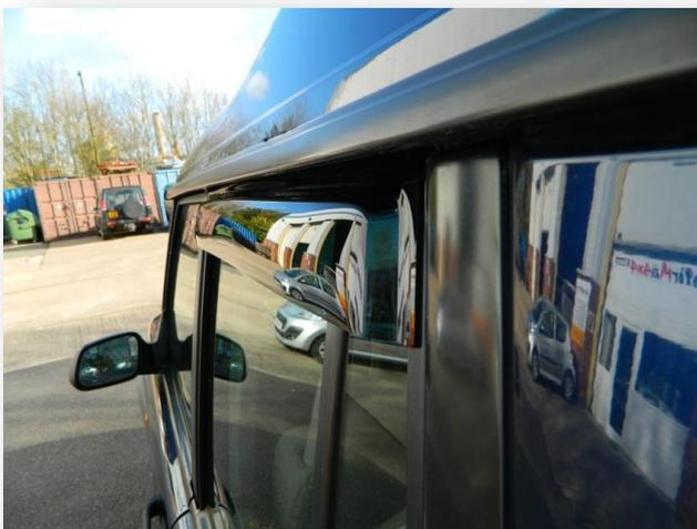
Rear deflectors should align perfectly with the door frame.
