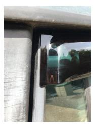
Rear deflectors should align perfectly with the door frame.
