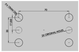
Once marked, position the external relocation plate over on the mount and check the marked position matches up with the holes in the plate. Once you are happy with this drill though the plate using a 10mm drill bit.
