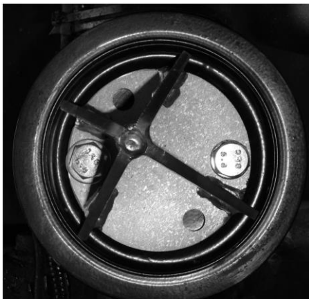
Image left is a top view of the cone fitted on the LH side of the vehicle, note which holes are used.
