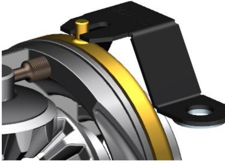
There should not be a gap between the two clamped surfaces.
