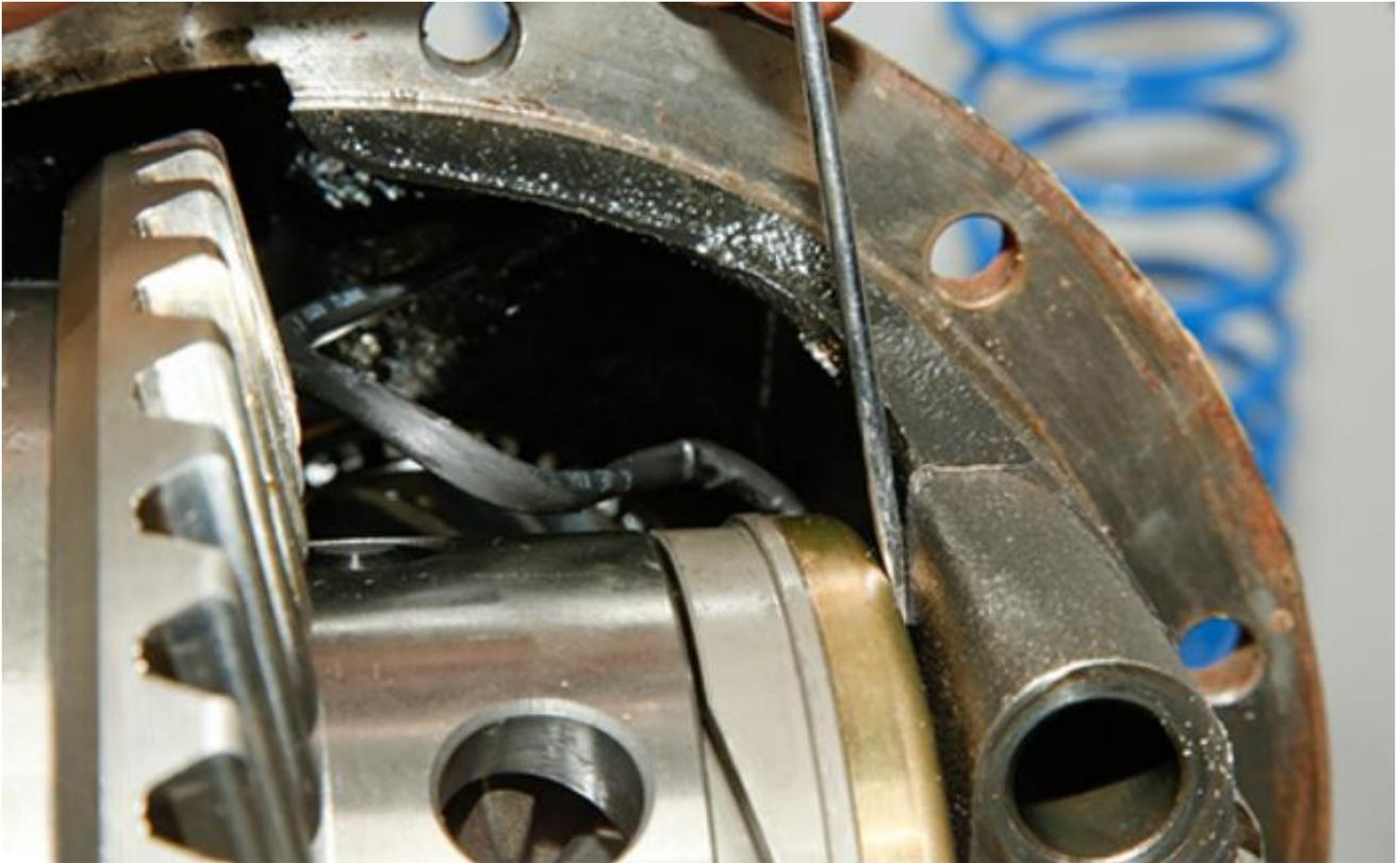
Position the electric cable and anti-rotation peg on the electromagnet to the top so they are visible when you fit the bearing caps.
