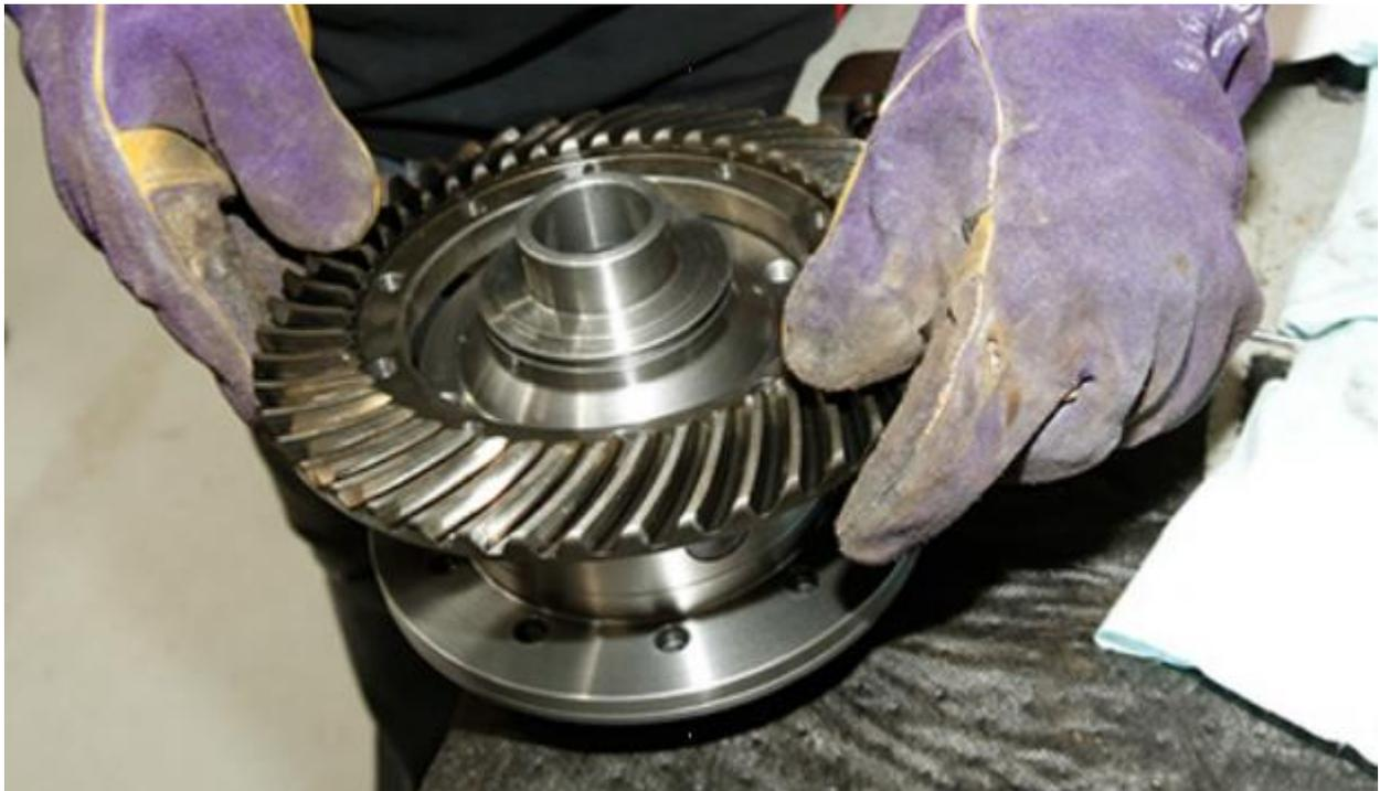
Position the crown wheel onto the E Locker center.
