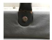
3. Remove the two screws that secure the plastic cover over the rear wiper motor.
