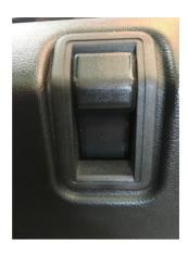
4. Remove the window winder handle by removing the "c" clip behind the cover:
