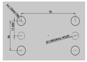
Once marked, position the external relocation plate over on the mount and check the marked position matches up with the holes in the plate. Once you are happy with this drill though the plate using a 10mm drill bit.
