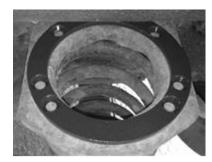
Mark the four holes on the outer edge of the ring. Drill these through with a 9mm drill.
