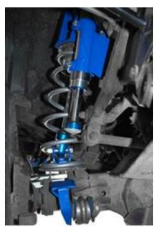
Fit the chassis plates with the vertical plate towards the back of the vehicle. Attach this using the two rear bolts only (M12x100 with washers) align the plate using the original bolts through the front holes and fully tighten the new rear bolts. Remove the front alignment bolts.
