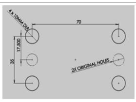
Once marked, position the external relocation plate over on the mount and check the marked position matches up with the holes in the plate. Once you are happy with this drill though the plate using a 10mm drill bit.
