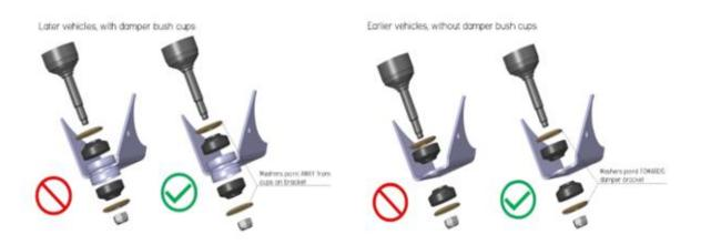
c. \*\*NOTE – Terrafirma TF2122 +5" shocks have pin top mounts instead of the conventional ring, this is to allow unrestricted articulation and movement of the mounting point. To allow these shocks to be fitted it is necessary to also fit TF519 extreme long travel rear top shock mounts that are simply bolted to the original mounting points. These are sold separately and not included with the shock absorbers.
