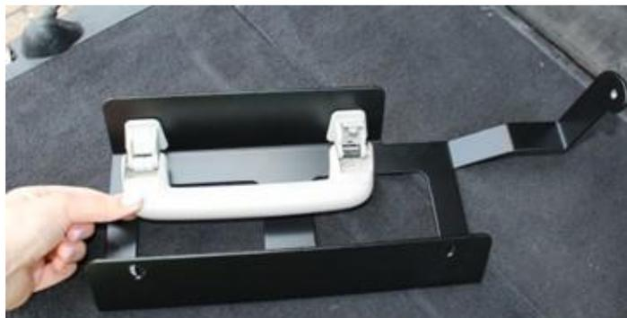
Offer the grab handles and brackets up to their original location before using the panhead retaining screws to secure them in place on both sides of the vehicle.
