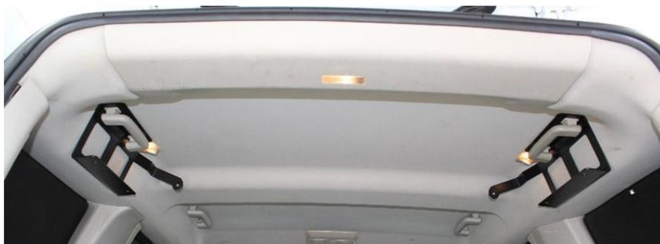
Open one of the passenger side doors, slide the rack in to the back of vehicle then lift the rack up and slide in to place so that it rests on the mounting brackets. This may be easier with an assistant but is not necessary.
