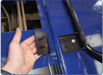
In the middle of the centre bar there are 2 mounting points, these should align with 4 pre-drilled holes in the seat base.
