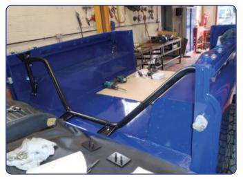
Once all the nuts/bolts and brackets are in position tighten up the nuts and bolts from the centre bar fixing points outwards to a torque of 40 newton metres.
