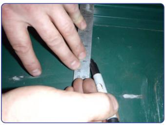
From behind the seats there is a vertical row of rivets which is the join of the wheel arch seam. Depending which side you are, mark a line to match the same position as that on the other side of the bulkhead. Tip - From in the rear tub measure from the centre of the rivet to the cut line you have already drawn and transfer these measurements to the front side of the bulkhead.
