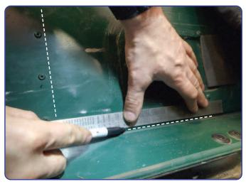
From behind the seats mark a cut line just above the lower part of the bulkhead across between the 2 wheel arches joining up to the 2 vertical lines you have drawn.
