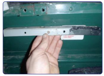
Along the top bar of the bulkhead there are 2 reinforcing pieces riveted in from underneath either side. Using a 5mm drill bit, drill out the rivets and remove these pieces.
