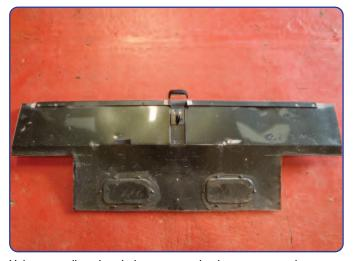
Using a small angle grinder or power hack saw, cut out the centre section of the bulkhead being careful not to cut over the ends of the cut lines and remove the centre section.
