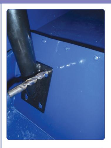
Fit the tube side brackets into position and secure at the top using the pan head bolts provided.
