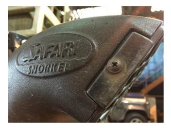
3. Attach the new stainless steel grill to the head of the Safari snorkel re-using the original screws.
