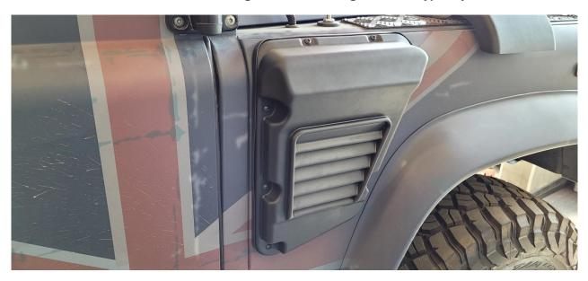
Remove the original plastic air intake vent.
