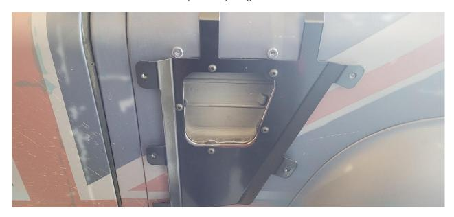
Starting from the bottom of the vent panel attach the rubber sealing strip and work around the vent until you meet the start, take care not to stretch the rubber. Cut off the excess length.
