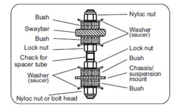
Grease bushing face and ID only Grease bushing ID only
