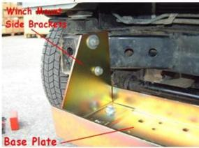
Photograph shows <u>vehicle</u> <u>without</u> winch in place and with <u>bumper</u> <u>removed</u>.
