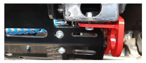
Loosely bolt the side plates to the inside of the chassis rails using the bolts for the lashing eyes through the recovery points. Refit the steering box support bracket bolt and the long M10 bolt from the fitting kit that secures the side plate opposite the steering box in the spare hole in the chassis rail.
