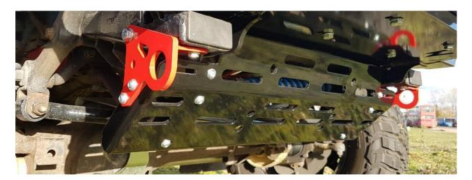
Offer up the guard to the two side plates and recovery points and loosely bolt together using the M8 button head Allen bolts, nuts and washers.
